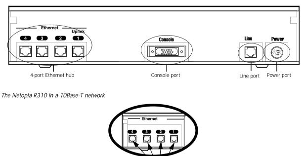
To connect your 10Base-T network to the Netopia R310 through an Ethernet port, use a 10Base-T cable with RJ-45 connectors.
